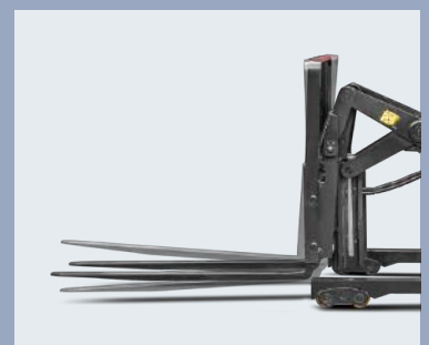
Mast tilting function is easy for entry in/out the pallet
