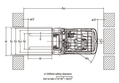
X: Load distance B: Length of load or forks which is longer
