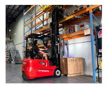
Designed to function optimally in incredibly tight working areas, the 3 Wheel Electric Counterbalance offers a lower minimum aisle width than most forklifts in its category.
