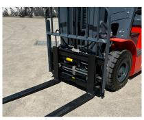
This 1.8T Lithium 4 Wheel Electric Forklift is equipped with a container mast with a low collapsed height, making it ideal for working in containers, under low doorways, and in heightrestricted warehouse environments.
